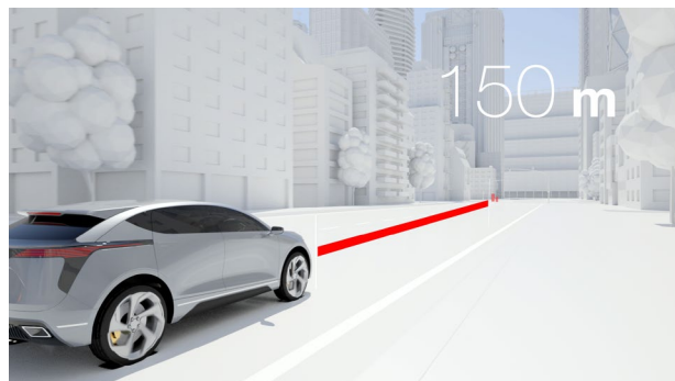
Magna’s ICON Digital Radar detects pedestrians up to 150 meters away
